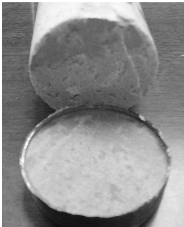
Figure 8. Baseplate Core Sample with Zinc Primer.
