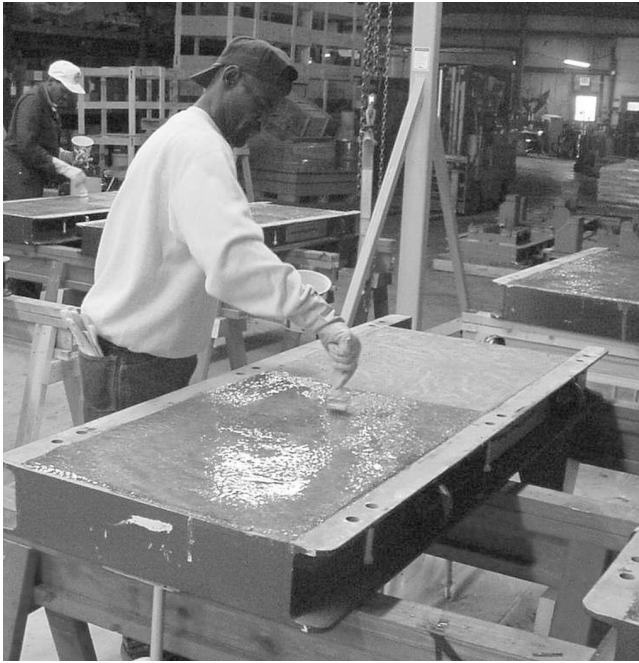
Figure 16. Epoxy Sealer for Cementitious Grout.
