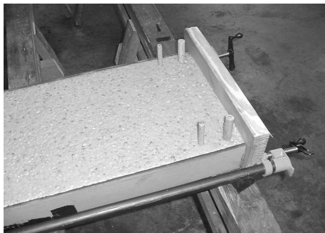
Figure 14. High Fill Epoxy Grout System.
