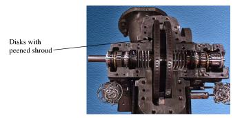
Figure 7. Photo of Small Turbine with Cover Removed Showing Rotor.
