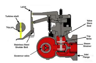
Figure 3. Illustration of Typical Steam Chest.
