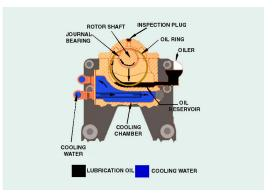
Figure 9. Ring-Oiled Lubrication.
