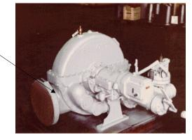
Figure 5. View from Exhaust End of Steam Turbine.
