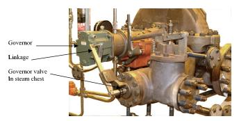
Figure 11. Turbine Controls.
