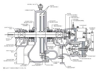
Figure 1. Cross Section of Typical Single-Stage Steam Turbine.
