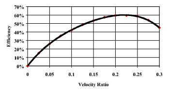
Figure 12. Typical Efficiency Curve for Single-Stage Turbine.
