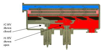
Figure 14. Hand Valve Illustration.
