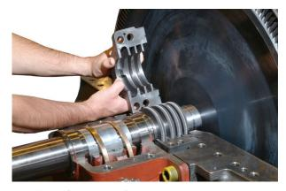
Figure 10. Carbon Ring Seal Arrangement.
