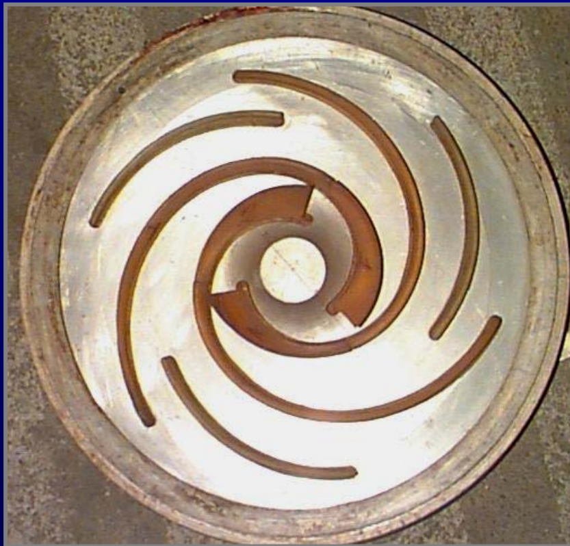
IMPELLER PATTERN WITH 3 PARTIAL VANES ADDED
