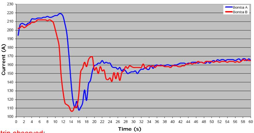
Electric Motor Current Behavior of A and B Pumps when Pump C is Tripped
