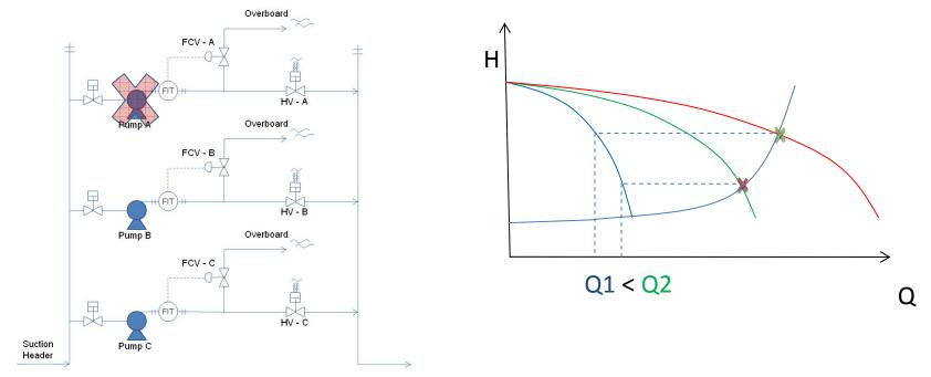
The increase in the outflow of the remaining pumps often reaches the maximum allowed outflow, as a result all pumps trip.
