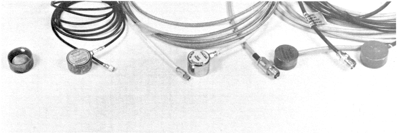
Figure 2. IFD Sensors: (l. to r.) Crystal Mounting, Boeing Design (N/A), Metrix Wide Range, HERCO, Acoustic Emission Technology.
