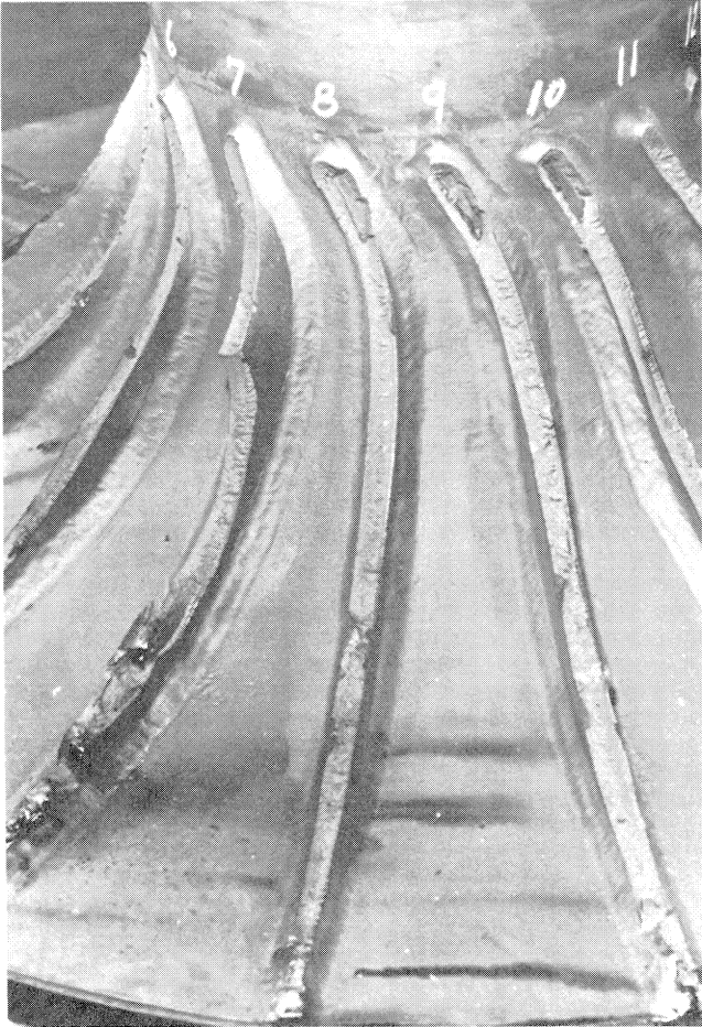
Figure 6. Open Impeller Showing Fracture Surfaces where Other Blades Separated from the Disc.
