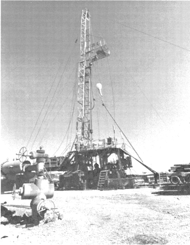
Figure 7. 150 Foot Tall Well Drilling Rig at The Geysers. The Rig is Portable and the Hinged Derrick is Self-erecting.
