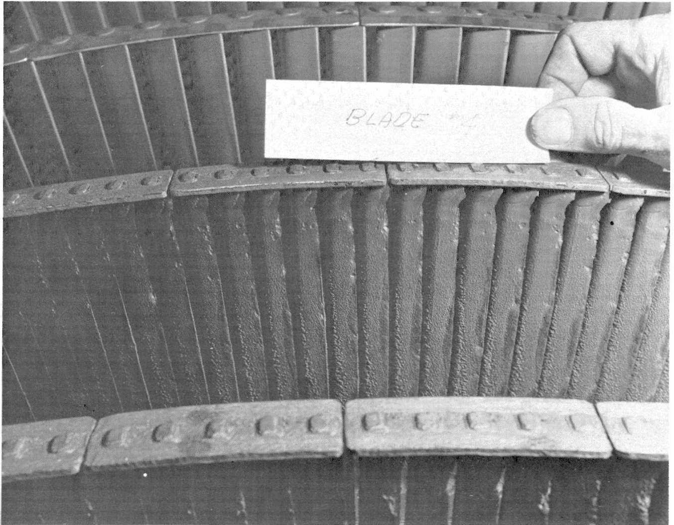
Figure 15. Geothermal Turbine Blade Erosion at The Geysers.
