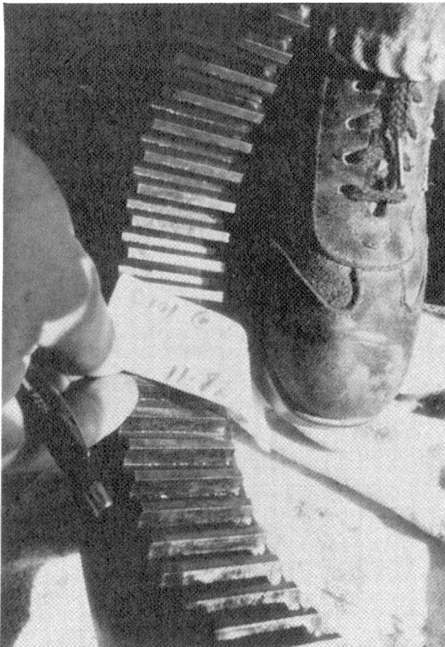
Figure 22. Compressor Side Coupling Shroud Gear Teeth Showed Excessive Wear for Only Nine Months of Service.
