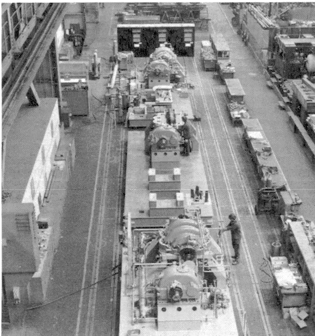
Figure 6. Refrigeration Compressors Being Assembled and Piped on Their Base Frames at the Supplier's Works.
