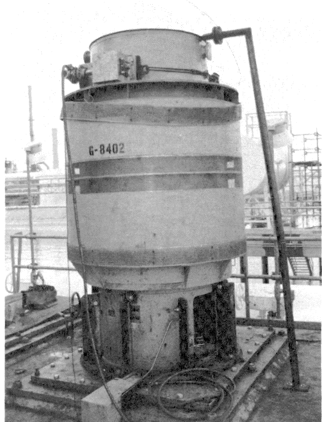
Figure 2. Variable Speed Shaker Mounted on the Motor.
