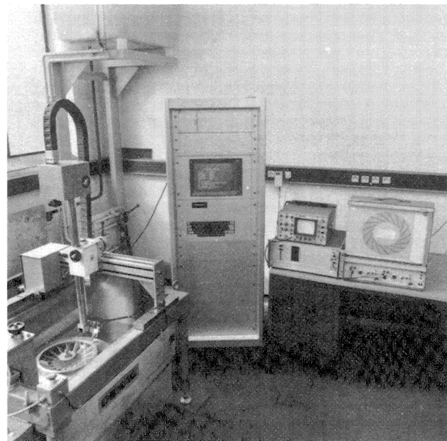
Figure 40. Ultrasonic Test Facility for Brazed Impellers.
