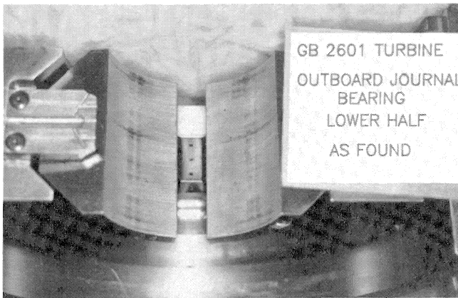
Figure 33. Lower Half of Governor-end (Outboard) Radial Journal Bearing After One Year of Service.
