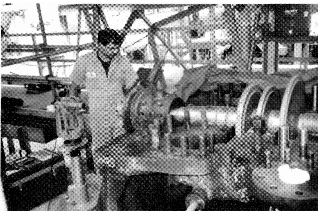
Figure 6. Optical Alignment with Mirror at Turbine Exhaust Shaft End.
