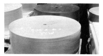
Figure 9. Rotor Laminations with C5 Core Plate.
