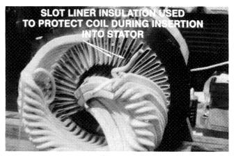
Figure 22. Use of Slot Liners Used to Protect Coils During Insertion into Stator.
