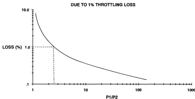
Figure 6. Loss in Available Energy Due to One Percent Throttling Loss.
