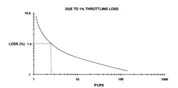
Figure 6. Loss in Available Energy Due to One Percent Throttling Loss.
