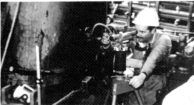
Figure 13. Technician Taking Vertical Readings.
