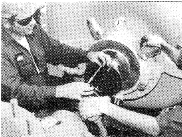
Figure 60. Distance Between Shaft Ends (DBSE) Determined.
