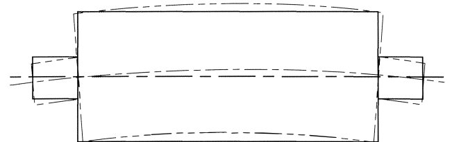
Figure 26. Rotor Bow Due to Uneven Cooling.
