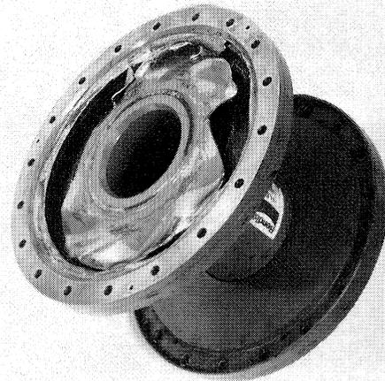
Figure 3. Diaphragm Buckling-Shear Failure Mode.
