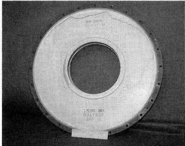
Figure 5. Circumferential Diaphragm Failure 300 Deg Arc.
