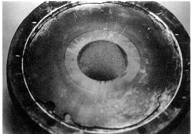
Figure 4. Diaphragm Failure Crack 90 percent of Periphery.
