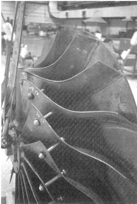
Figure 5. Open-Inducer Impeller with Zig-Zag Damping Pins.
