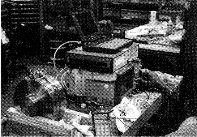
Figure 4. The Probe Calibration Sample and Clamp (Lower Left), Thermocouple Reader (Lower Middle), Oscilloscope (on Table) with Pulser/Receiver and Computer on Top.
