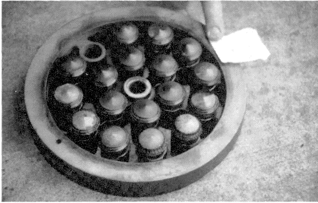
Figure A-2. Poppet Valve with Failed Poppets. (Note the poppets at locations 5:00, 6:00, and 7:00. You can see where springs have "rolled over" the head of the poppets, causing indentations. Poppet at location 11:00 is missing.)
