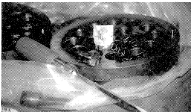
Figure A-3. Poppet Valve Cover Showing Damaged Springs. (Springs had extended and gotten under the heads of the poppets.)
