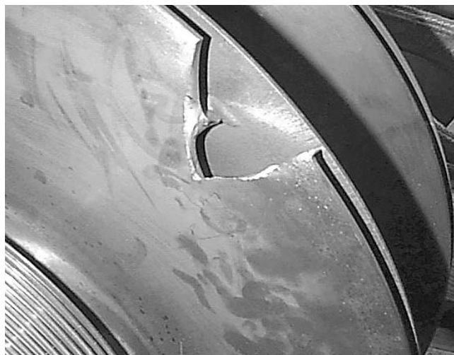
Figure 10. Damage at Tip of Cutback Impeller for Case B.
