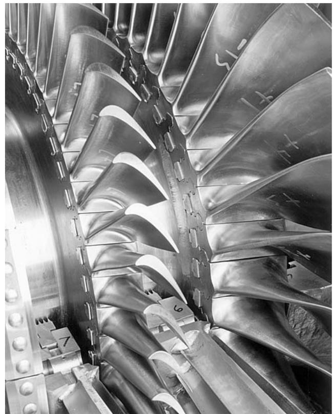
*Figure 12. Low-Pressure Titanium Freestanding Blades.*
