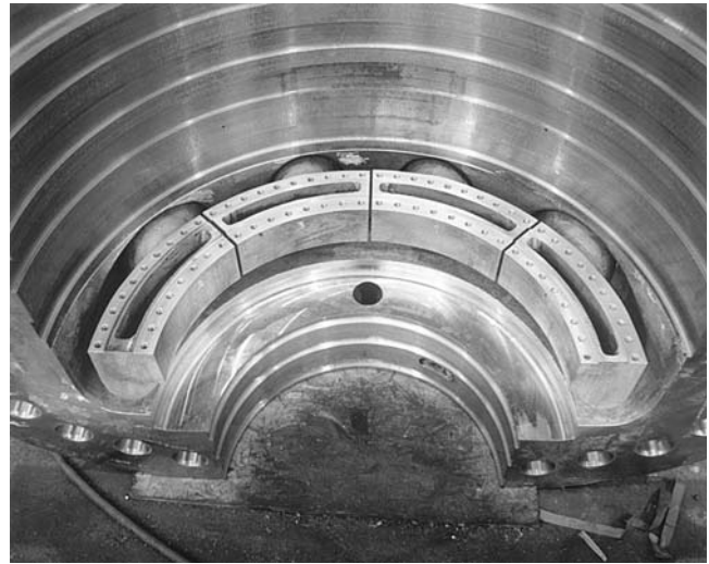
Figure 9. Nozzle Bowl Passages in Upper Half of Main Casing.
