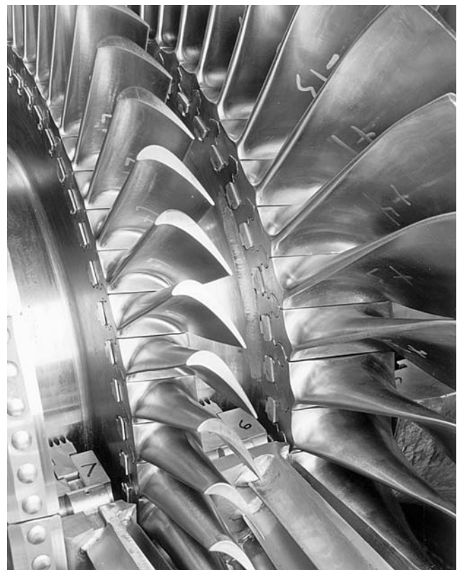
Figure 12. Low-Pressure Titanium Freestanding Blades.
