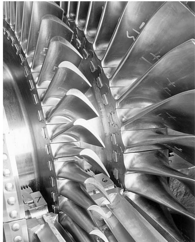
*Figure 12. Low-Pressure Titanium Freestanding Blades.*
