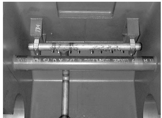
Figure 21. View of Inside of Gearcase Cover Showing Tie Bar Installed.
