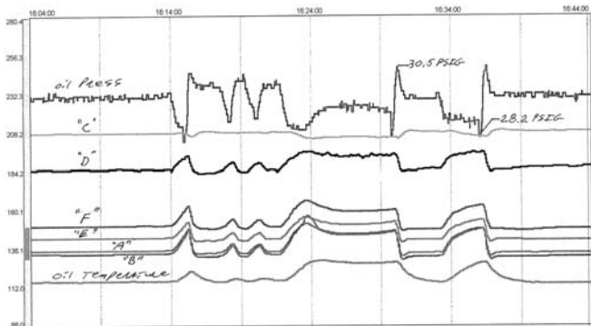
Figure 4. Oil Temperature as Seen in Plant Control Room During Oil Temperature Test 1.
