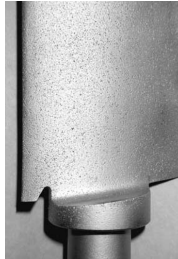
Figure 3. Corrosion Pitting on 410 Stainless Steel Inlet Guide Vane.
