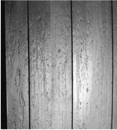
Figure 6. Corrosion of 4140 Alloy Steel Balance Piston Region.
