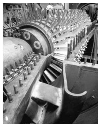
Figure 8. Upgraded Rotor Assembly Utilizing Titanium Alloy and C450 Blades, and a Coated Rotor Body.
