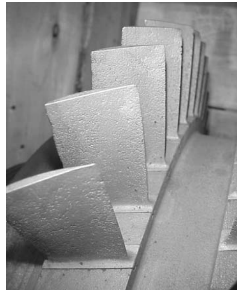
Figure 4. Corrosion Pitting on 403 Stainless Steel Rotor Blades.
