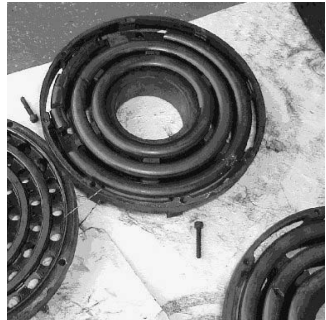
Figure 14. Damaged Suction Valves.
