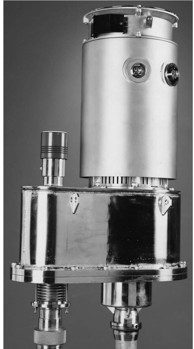
Figure 3. Helium Turbocompressor. (Courtesy, Fermilab Visual Media Services)
