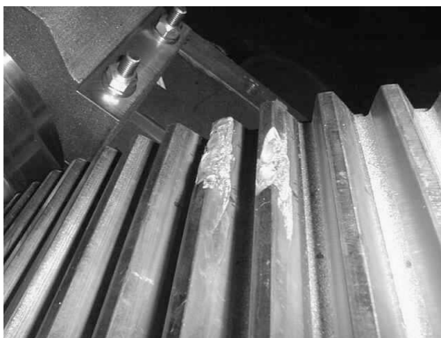
Figure 11. Local Damage on Gearbox Teeth.
