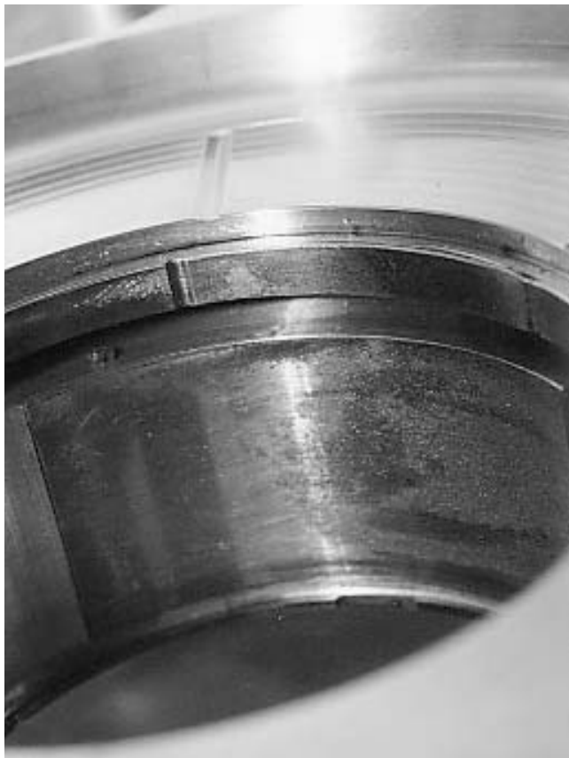
Figure 16. Bearing Surface Showing Pitting Damage.
