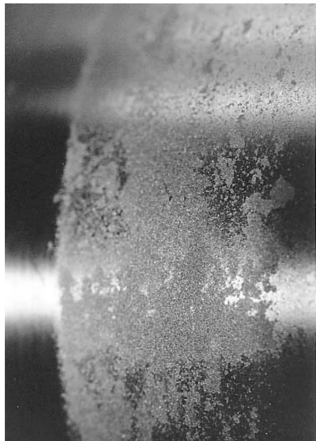
Figure 17. Shaft Journal Surface Showing Both Pitting and Deposition of Babbitt from Bearing to Shaft.
