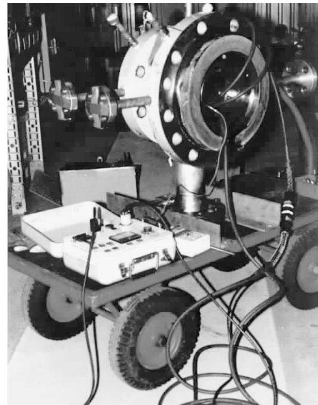
Figure 14. Turboexpander Bearing Housing Degaussing Setup.
