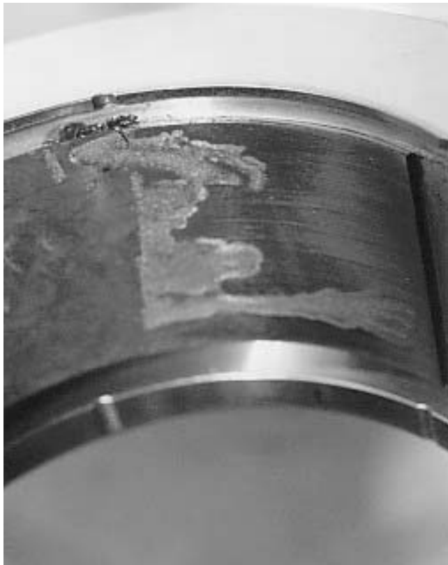
Figure 15. Bearing Surface Showing Bearing Damage Due to Pitting.
