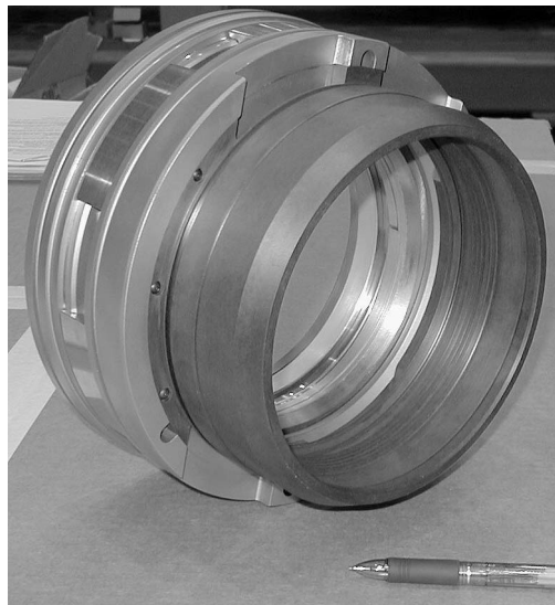
Figure 5. Inboard View of Upgraded Oil Sleeve Seal Cartridge Showing Thermoplastic Labyrinth Seal (Front) and Contaminated Drain and Vent Slots
