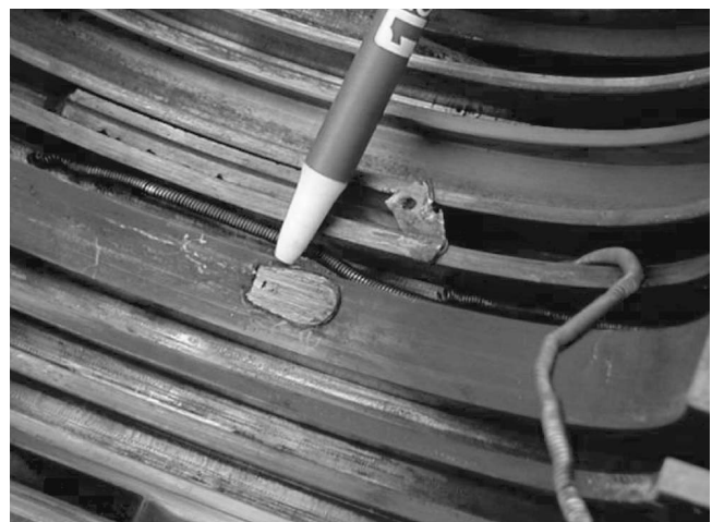
Figure 9. Antirotation Tab "Smeared" onto Seal Housing.
