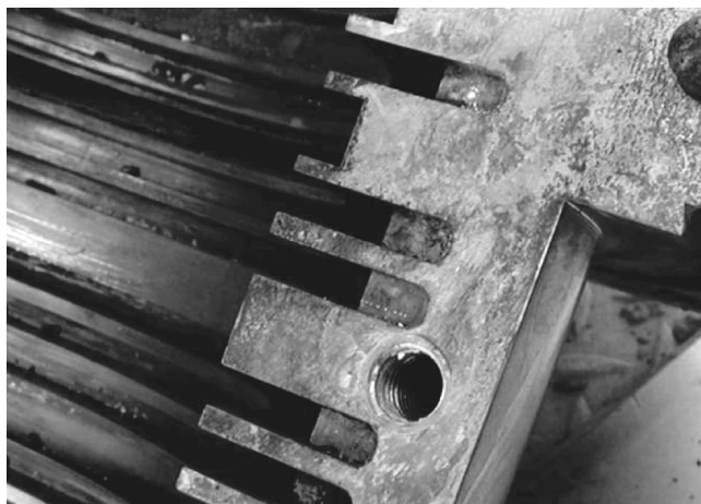
Figure 10. Seal with Slots for Antirotation Tabs.
