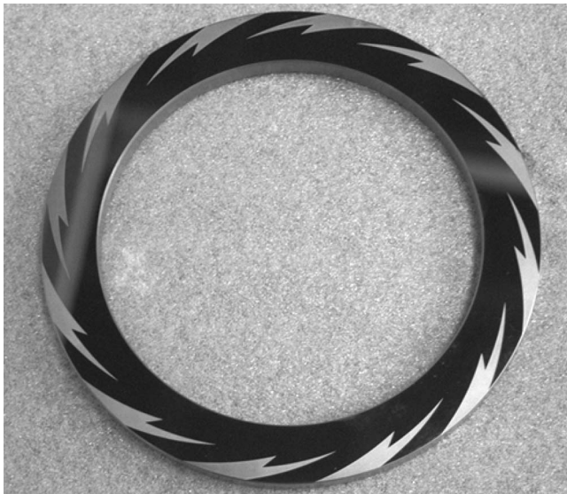
Figure 3. Grooves in Gas Seal Mating Ring.
