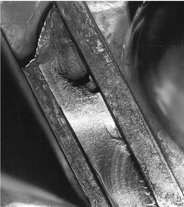
Figure 10. Closeup of Low Cycle Fatigue Failure Shown in Figure 9.
