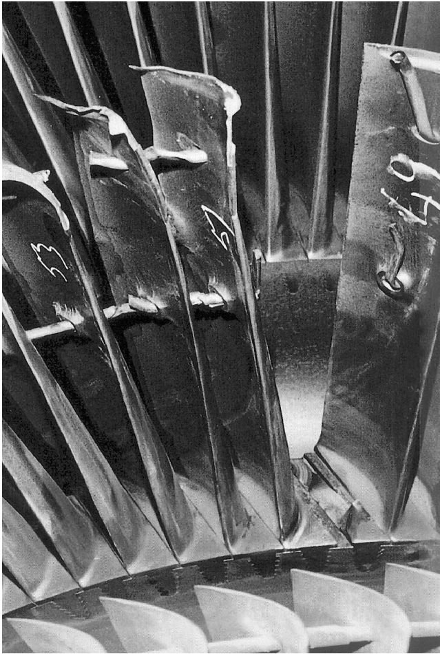
Figure 9. L-1 (Next to Last) Stage Blade Failure at Base of Airfoil Due to Low Cycle Fatigue.
