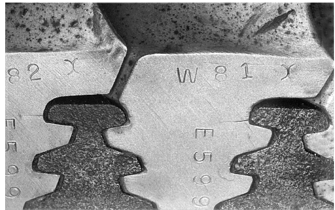
Figure 27. Corrosion Fatigue in L-1 Blade. (Crack initiation and propagation can be seen in first hook (serration) of two blade roots shown.)
