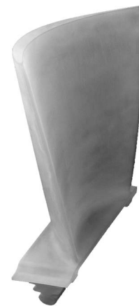
Figure 14. Prototype of Redesigned Rotor.
