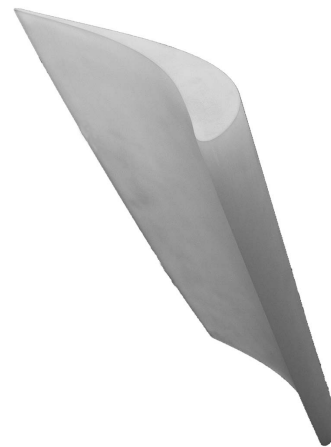
Figure 13. Prototype of Redesigned Stator.
