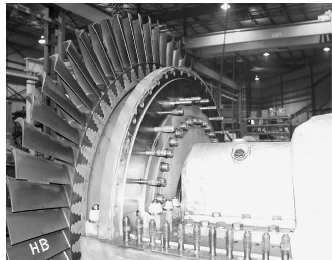
Figure 3. Cross Section of OEM and Upgraded Seal Housing Designs with Photograph of Installed Upgrade.
