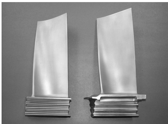
Figure 8. Comparison of Original Rotor Blade (Left) and Upgraded Design for Higher Operating Temperatures (Right).
