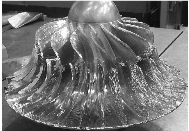
Figure 24. Impeller Side View—after Heavy Erosion Damage.
