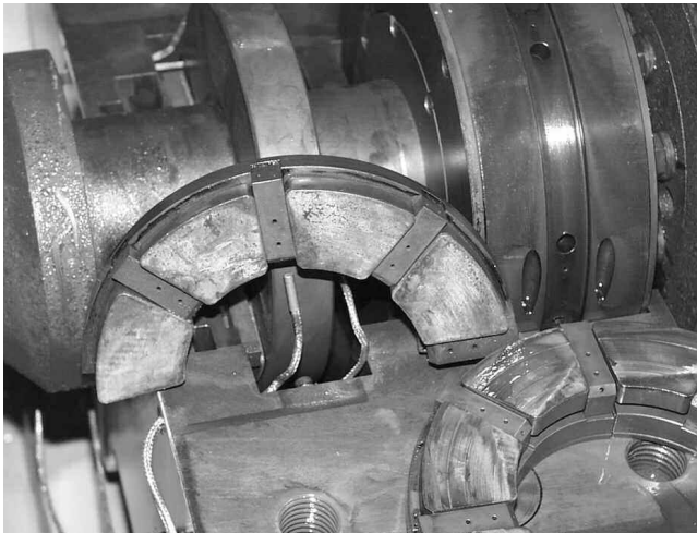
Figure 21. Thrust Bearing Heavy Babbitt Corrosion Due to Oil Contamination.
