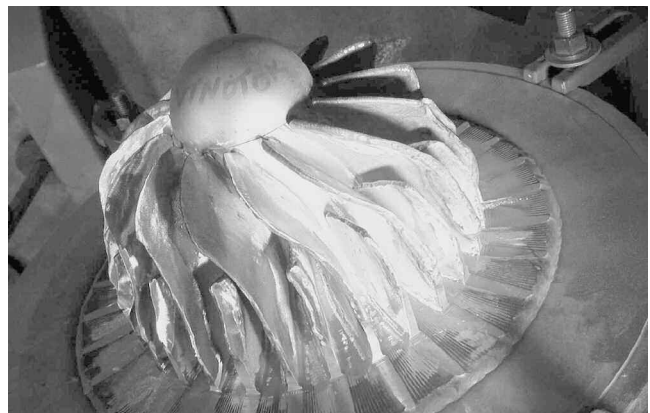
Figure 26. Impeller in Repair via Coupon Method.
