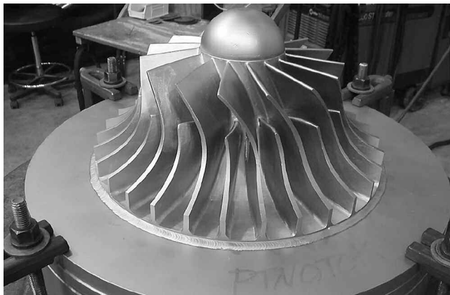
Figure 27. Nearly Finished Repaired Impeller.
