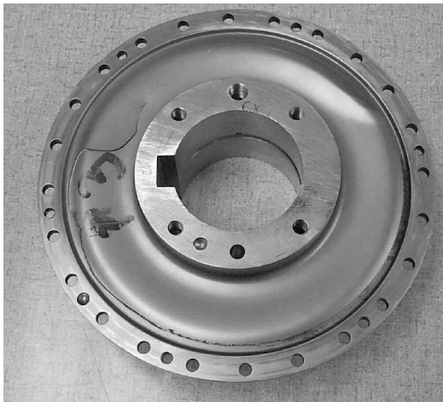
Figure 56. Reduced Moment Diaphragm Failure from Angular and Axial Misalignment.
