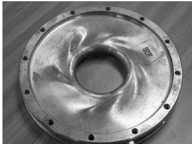
Figure 59. Diaphragm Torque Overload.
