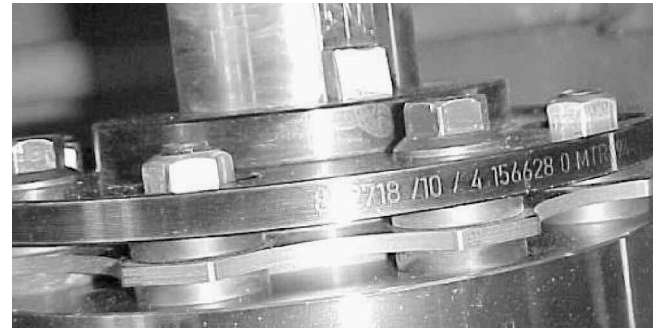
Figure 30. Disc Coupling—Note Alternating Attachment Fasteners.
