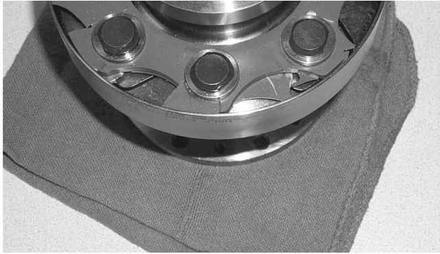
Figure 39. Outer Disc Failure—Note Interlocking Flange Back-Up in Case of Total Failure.
