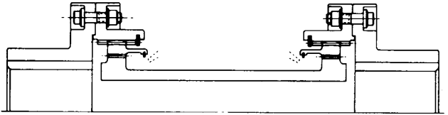
Figure 17. Marine Style Gear Coupling Generally Continuous Lube but Also Used in Pack Lubed Configurations (Accessory Drives for Gas Turbines).
