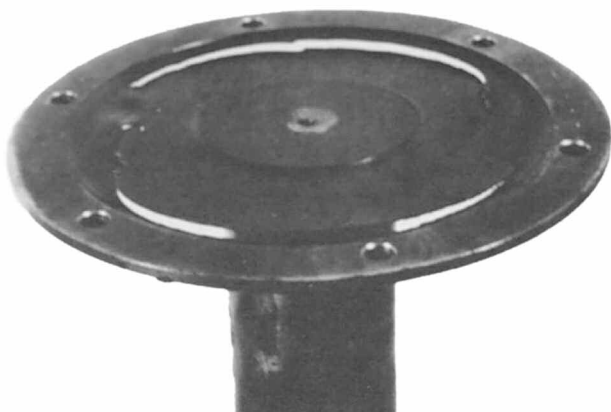
Figure 57. Marine Style Diaphragm Failure from Angular and Axial Misalignment (A).
