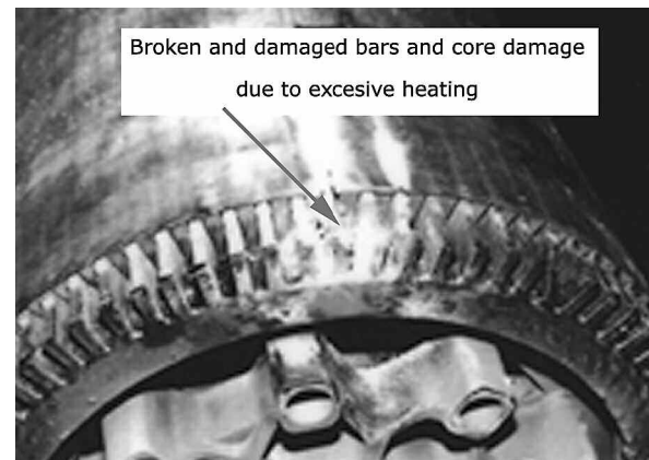
Figure 10. Food Mixer Motor—Broken Rotor Bars.
