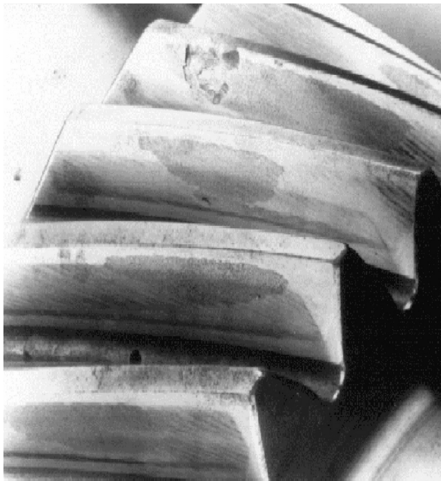
Figure 7. Micropitting. (Courtesy ANSI/AGMA 1010-E95, 1995)
