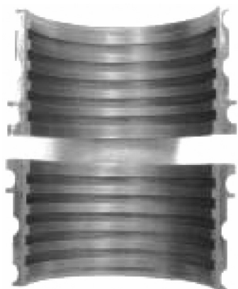
Figure 19. Nickel Graphite Packing Case Seals Prior to Run.
