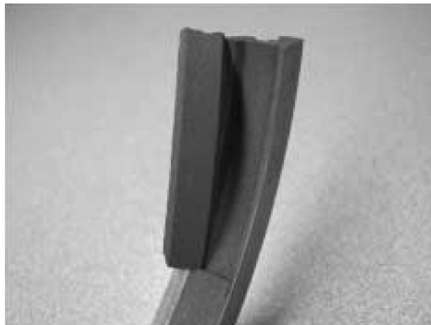
Figure 6. Delamination of Nickel Graphite Seal Due to Reaction of CO with Ni.
