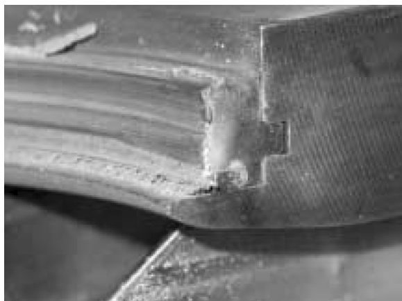
Figure 5. Damage to Nickel Graphite Impeller Seal.
