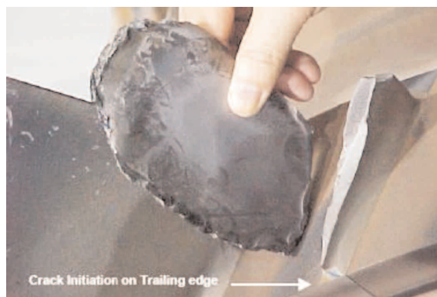
Figure 12. Failed Axial Blade. Crack Initiated on High Pressure, Trailing Edge of Blade.
