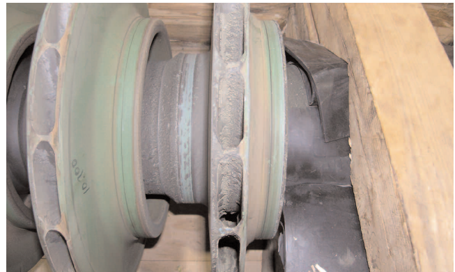
Figure 16. Synthetic Natural Gas Compressor Rotor. Note Fouling in Impellers. Monitoring Compressor Performance Helps Track this Condition and Aids Scheduling of Maintenance.
