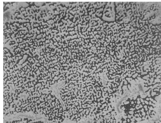
Figure 20. Change in Gamma-prime Morphology, 1000X. Large Amount of Agglomeration.
