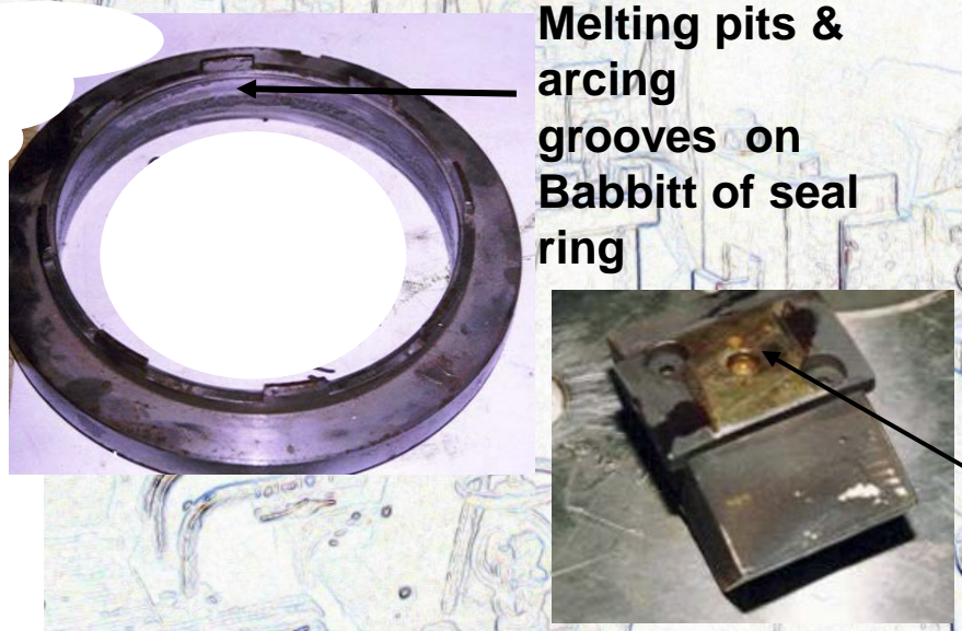
Spark tracks on back seating area of journal bearing pad
