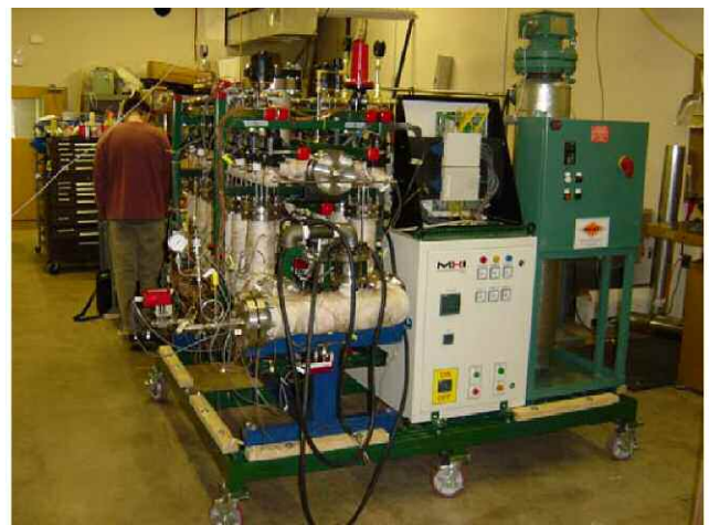
Figure 2. LPP Liquid Fuel Vaporizer Skid Used for Gas Turbine Burner Testing at Elevated Pressures.
