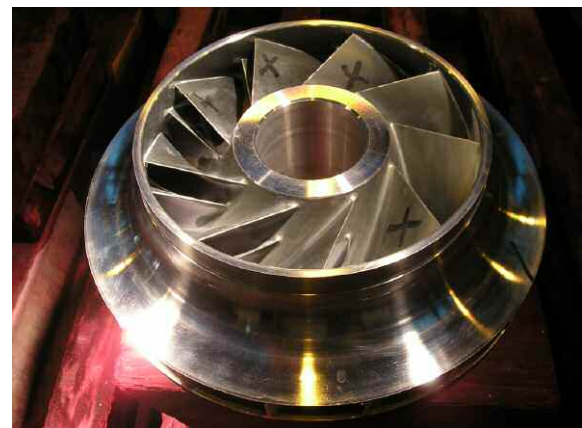
Figure 21. Impeller of Third Generation for Flow Coefficient 0.127.
