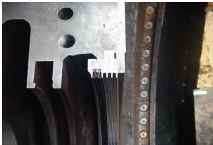
Figure 4 Bearing No1, lower half of labyrinth seal and non-metallic brush seal. Bristles are black colored.
