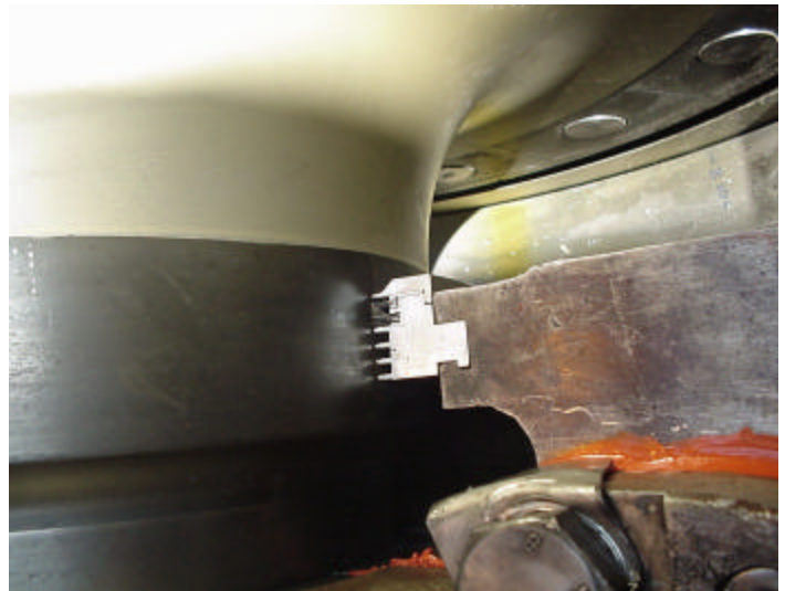
Figure 6 Brand-new non-metallic brush seal.
