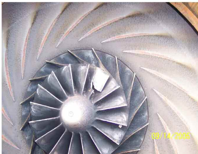
Figure 3. SCC Failure Due to Chloride and Sulfur in Air Stream.
