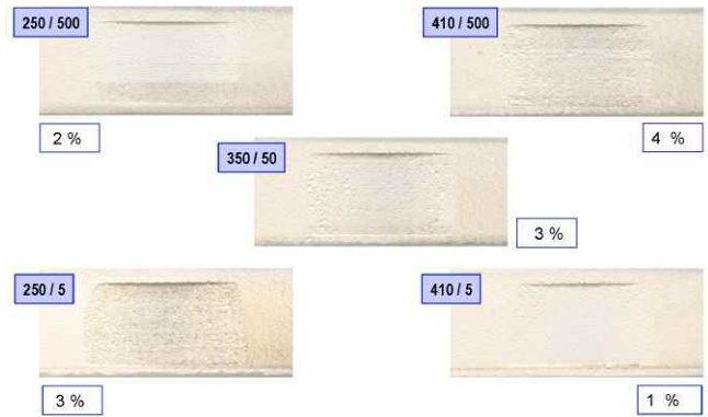
Figure 16. Abradability Results for a Porous (43 Percent) YSZ Ceramic Abradable at 1100°C (2010°F) under Rig Set Conditions as Indicated. Blade Wear as a Percentage of Total Incursion.
