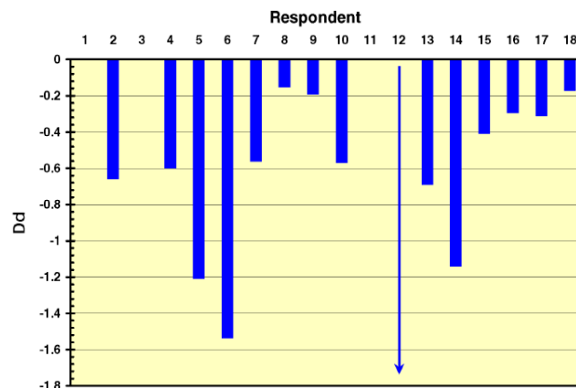
Figure 15. Labyrinth Seal Impact on Predicted Log Dec.
